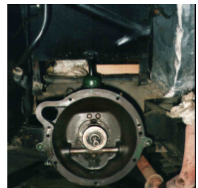
Hole in the bell-housing for the starter motor shaft.
