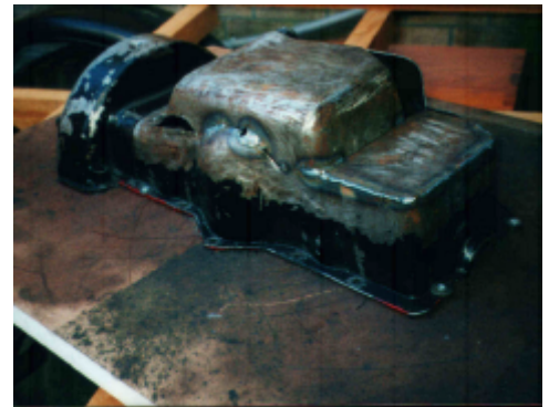
Part-way through the welding process.
