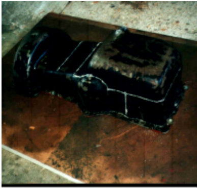
Original sump marked-up for cutting.
